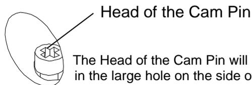
The Head of the Cam Pin will be visible in the large hole on the side of the joining board.
