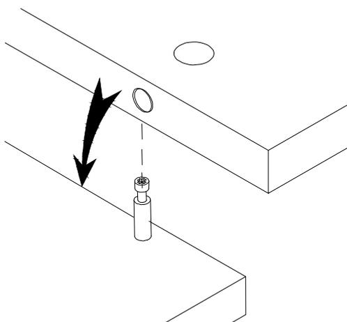
Now fit the hole in the edge of the joining board over the Cam Pin.
