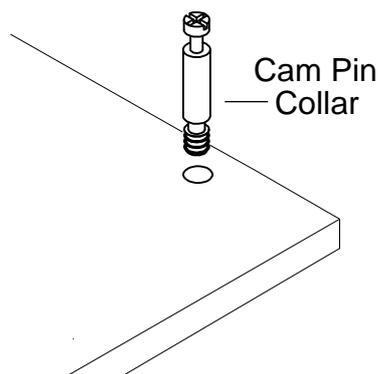
The Cam Pin is inserted into the flat side of a board, it is important that: The cam pin is kept vertical and is not put in on an angle.
