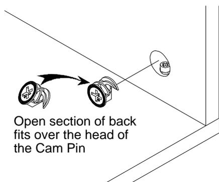
Open section of back fits over the head of the Cam Pin
